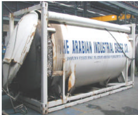
Major failure of nitrogen tank
